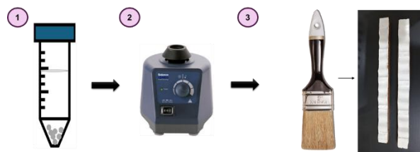
Figure 1. Formulation (1), particle dispersion (2) and coating (3) of the photocatalyst onto the red cooked clay tiles.
