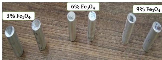
Figure 2. Wear test specimens of Al-Fe 3 O 4 composites with varying reinforcement contents (3%, 6%, and 9% Fe 3 O 4 ).
