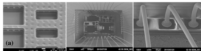
Figure 6. Process E. SEM (a) image of chip etched with Silox Vapox III, detail of the proof mass orifices allowing the etchant penetration. Process E. (b) SEM image of packaged FG MOS–MEMS inertial sensor, and (c) bonding wires, after post–processing.
