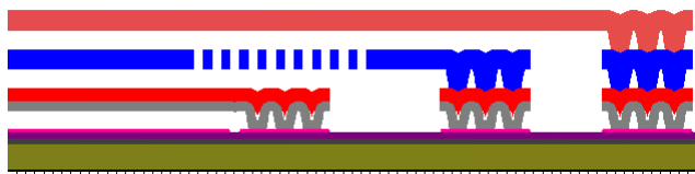
Figure 5. Lateral view from SUMMiT V final model of the movable membrane and rigid backplates.
