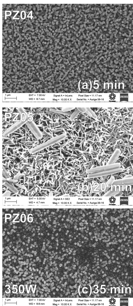
Figure 3. Scanning electron microscopy images of the ZnO nanowires grown on PET substrate at 350 W and with a heating time of (a) 5 min, (b) 20 min and (c) 35 min.
